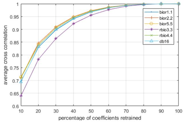
Figure 4. Selection of optimal mother wavelet for vibration bearing signals
