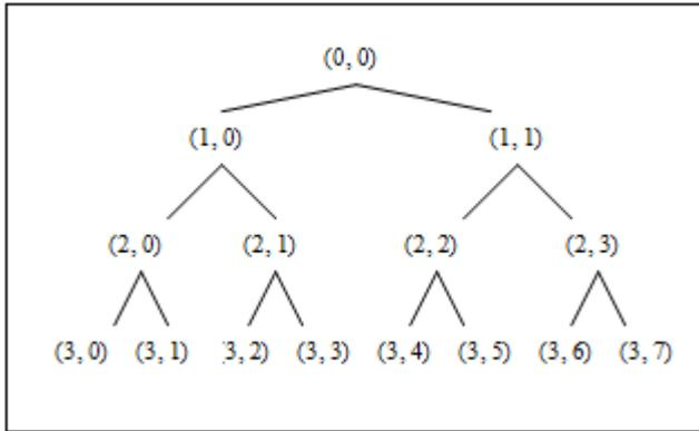
**Figure 2. The tree of wavelet packet decomposition. Each doublet (k,i) represents the depth (k), and the number (i) of the nodes.**
